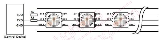
In the practical application circuit, in order to prevent the instantaneous high voltage generated by the hot plug of the product during the test from damaging the IC internal signal input and output pins, the protective resistors should be connected in series at the signal input and output terminals. In addition, in order to make the IC chips work more stably, a decoupling capacitor between the lamp beads is recommended;
