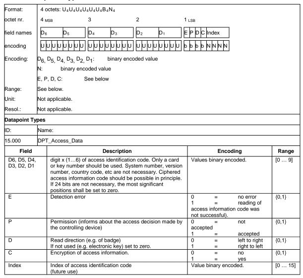
EXAMPLE 1: Transmission of the access identification code "123456", without error indication, permission accepted, badge read from left to right, no encryption and index 13.
