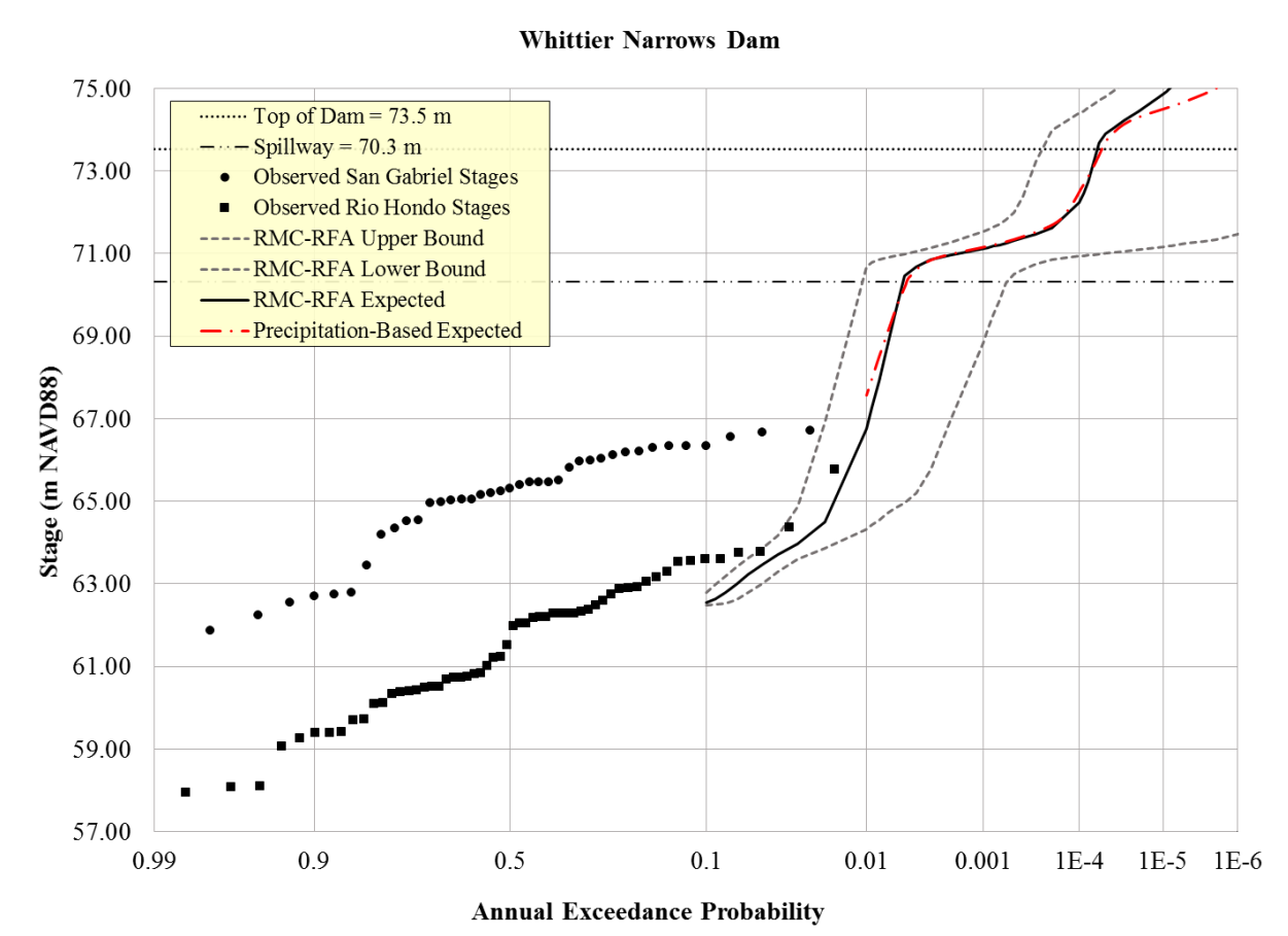
Figure 9. Comparison of stage-frequency results for Whittier Narrows Dam using RMC-RFA and regional precipitation-frequency analysis. The figure shows the 90% confidence intervals and the expected probability curve produced by RMC-RFA. Only the expected curve from precipitation-frequency based results is shown.
