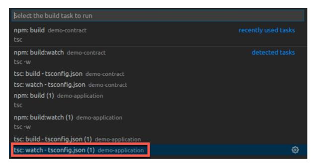
After a few seconds, the application will have been built and the compiler will enter '*watch*' mode, which means that any changes to the source will cause an automatic recompilation. Using watch mode is useful as it means you do not have to force a rebuild each time you make a change.
